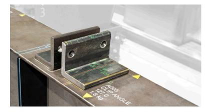
The LayoutMaster combines your 3D CAD details with color laser technology and AGT's award-winning Cortex software to project all the information needed to assemble parts on a beam quickly and precisely.
