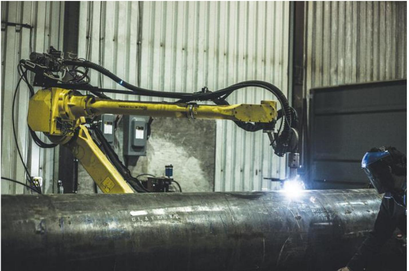
Groupe Gravel's robot workcell performs plasma cutting and welding on large workpieces at the company's Quebec facility.
